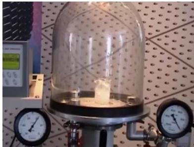
Video view shows it appears that the water in a glass that is inserted into the vacuum desiccator appears to boil when the desiccator space is exposed.
